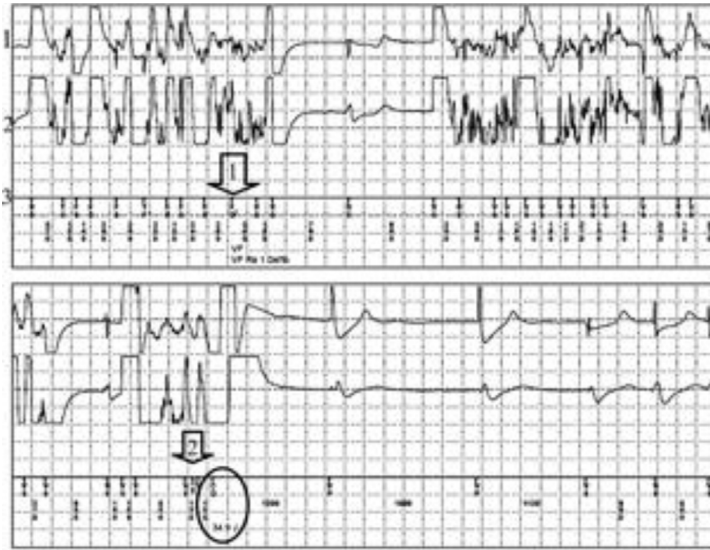
Fig. 11. Intraoperative EMI from monopolar electrosurgery leading to an inappropriate ICD shock. The electrogram demonstrates that a short burst of monopolar electrosurgery at an inopportune time caused the ICD to misdiagnose EMI as a malignant rhythm and deliver a 34.9-J shock. Trace "1" (top panel) reports the RV signal from the RV tip to ring electrodes. Trace "2" reports the RV signal collected using the RV ring electrode and the ICD "can." Trace "3" reports the ICD interpretation (marker channel) of the events (see legend below). At downward arrow "1," the ICD determined the aberrant signal persisted long enough to declare a ventricular fibrillation event "FD" and charge the capacitor in preparation for shock. ATP while charging was not delivered owing to several short RR intervals preceding charge initiation (this ICD will not deliver ATP while charging when any RR interval in the 8 preceding RR intervals before the VF detection is <240 milliseconds). "CE" downward arrow "2" marks the end of capacitor charging and the start of VF reconfirm. Then, a very brief EMI event caused the 34.9-J charge delivery ("CD"). Because the EMI ("VF") stopped, the ICD classified this shock as successful termination of VF. The lack of EMI right after VF was declared too short to abort this event given the patient's native heart rate of about 80 bpm. CE, charge end; CD, charge delivered-cardioversion/defibrillation pulse; FD, VF detection; FS, VF sense; TS, VT sense; VP, ventricular pace; VS, ventricular sense.
